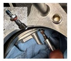
Put a dab of grease on screw head to keep screw attached to socket. Apply blue thread locker to screw. Install new supplied gasket and carefully start screw into case threads.
