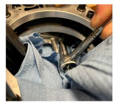
Loosen jet mounting screws to the end of their threads, but do not relieve pressure on screw.
