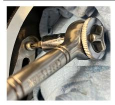
Check screw thread depth by installing screws without the jet. Verify that the screw threads in far enough to properly clamp the jet in place.
