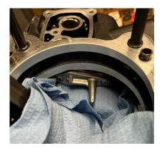
Pack area around cool jet with clean towels to prevent dropped screws from entering crankcase.
