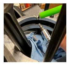
Place small magnet on screw when removing socket and screw together.
