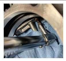
Repeat for second screw. Use inch-pound torque wrench and tighten screw to 35 inch-pounds. Repeat for the other cylinder.
