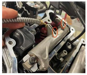
Before starting the engine, cycle it in short 10 second bursts using the starter with the spark plugs out but grounded. Add several squirts of **Spectro Motor-Guard Break-in oil** on the valve springs, rockers, and valve stems during these non-firing cycles with the pump oiler can before and during each of the 10 second "non-firing rotation" cycles. Watch for bubbles, then oil flow through the ports and channels on top of the rocker arms shown above in the red circles.
