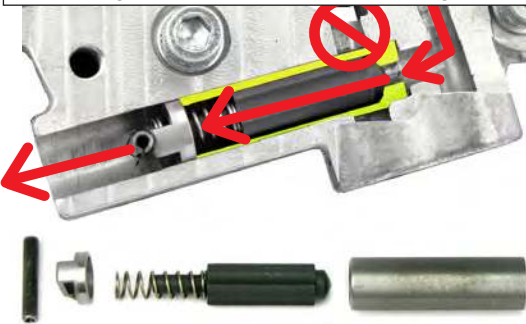
Cam Plate Cutaway with #620-103 Bypass Valve Fluted Design of Needle Allows Oil Flow Through Valve
