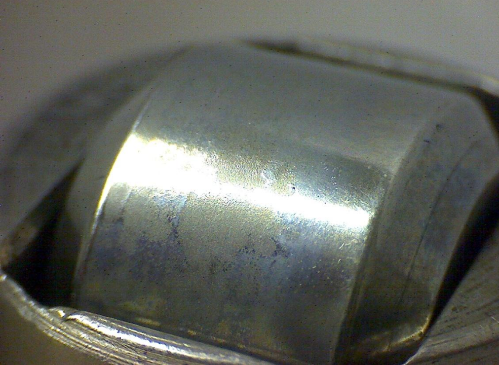
Material Transferring from the Roller onto the Camshaft
