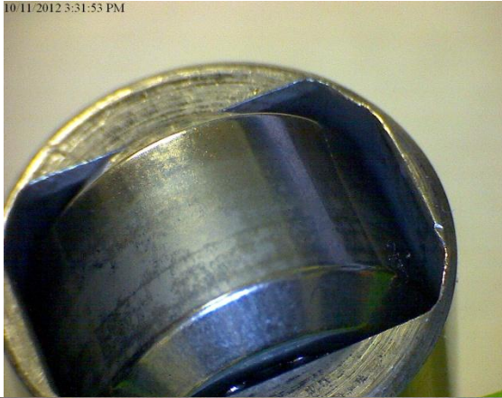
Material Transferring from the Roller onto the Camshaft
