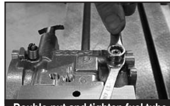
Double-nut and tighten fuel tube in place
