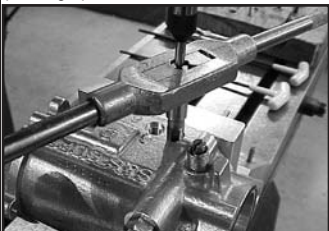
Tapping bowl vent for fitting
