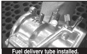
Fuel delivery tube installed.
