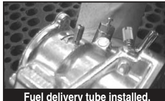
Fuel delivery tube installed.
