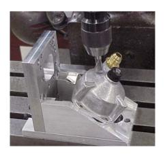
Secure float bowl to fixture using the 3/8"- 16 flange nut and threaded rod provided using the 35 degree slope. Clock (rotate) bowl as needed.
