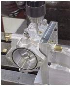
Using the two **#10-24** cap screws provided, secure the Carb body at bowl surface to fixture through the two holes marked 'B'.
