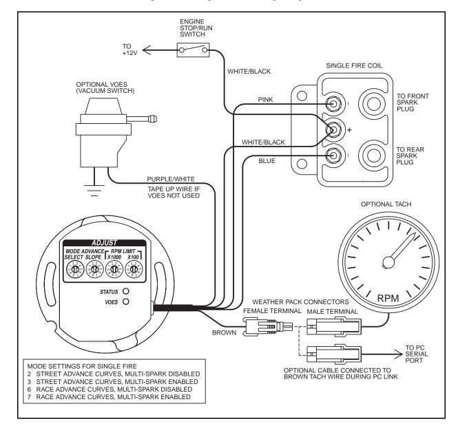
Figure 5 - Single Fire Wiring Diagram
