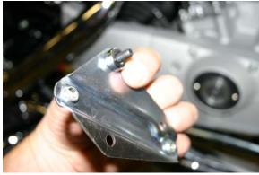
Place the filter element over the stanchions and install the cover bracket to the stanchions (the spacer goes between the element and the cover bracket). Leave the first screw loose and install the other two screws with spacers. Tighten the screws.
