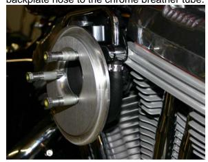
5. Locate the (3) Torx head screws and spacers supplied and Apply blue Loctite® to the screws. Insert a screw through the air cleaner cover bracket, and a spacer over
