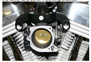
2. Place a sealing washer on both sides of the breather tube banjo fittings and install the chrome breather tube with the hose nipple on the front head using the banjo bolts supplied (be careful to center the sealing washers during tightening; use blue Loctite®). Do not overtighten.
