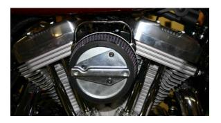
Re-install the air cleaner cover using the original mounting hardware (use blue Loctite®). Optional: Use an adhesive to attach the rubber seal trim to the cover for a finishing touch.
