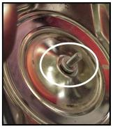
14. Locate the supplied A/C cover washer. From *inside* the cover, place the supplied washer over the cover bolt. Apply blue threadlocker on the threads of the bolt and install the cover assembly onto the air filter element.
