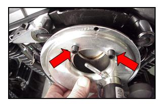
7. Insert supplied gasket between backing plate and throttle body. Apply blue threadlocker to threads of (3) supplied air filter stanchions and install. Tighten stanchions to 120-140 in/lbs.
