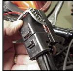
10. Carefully push the black housing cover locks of the ECM connector in to release the housing cover. Note there are (4) rows of terminal ports in the harness housing, (2) rows of 16 ports and (2) rows of 20 ports, each row has a starting number to identify the port number on the wire entry side (1<sup>st</sup> row [1-16] not used). You will be inserting (2) wires from the NADS harness into two unused ports that have sealing pins in them which must be removed before wires are added.
