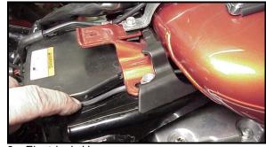
9. Electrical Harness Installation: Remove left side frame cover and remove the ECM fuse. Disconnect the negative battery cable. Carefully disconnect the wiring harness connector from the ThunderMax.
