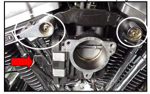
4. Install supplied breather spacer chrome caps onto the breather 'S' hoses and install the hoses to the breather bolts.
