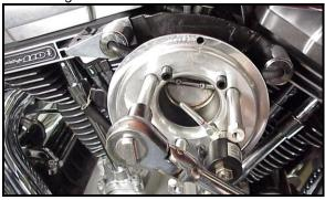
8. Plug two-wire harness connector into NADS solenoid attached to backing plate. Route remaining harness up to frame backbone, under fuel tank to ECM area under seat as shown.
