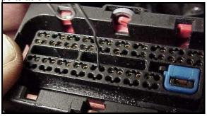
From the other side of the connector, remove the seal pin from port #26. Remove the unlocking clip or tool from the terminal side.
