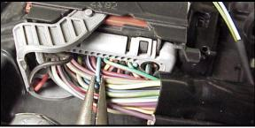
Install the white wire with black tracer into port #26. Bottom the terminal into the chamber then gently tug on the wire to verify that it has locked into place. Repeat this process for the yellow wire with black tracer into port #47.
