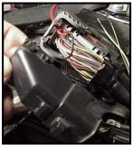
11. Snip wire tie holding harness to connector housing. Remove the green terminal lock pin from the housing using a small screwdriver (lock has one short, one long leg; note orientation).
