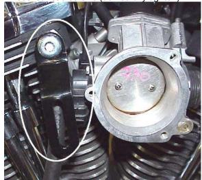
13. Apply blue Loctite to (3) 1/4-20 x 3/4 Torxhead socket screws and install backplate to
