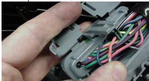
6. Re-install the connector retainer. Position the wires of the nitrous harness so that they exit the strain relief along the same path as the OEM wires. Close the halves of the strain relief around all the wires.
