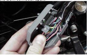
4. Depress the tabs on the connector retainer (clear plastic) and remove it from the connector.
