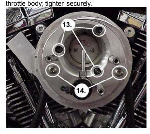
14. Attach backplate to support brackets using 5/16-18 bolts, nuts and washers provided. Use shims provided to fill any gap between bracket and backplate so that there is no stress or binding between the bracket and backplate while tightening (brackets may be bent slightly to ensure even alignment with backplate). Tighten the 5/16-24 sockethead screws securing the brackets to the banjo bolts.
