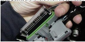
5. Locate positions 9 and 32 on the "wire side" of the connector. On the nitrous harness, insert the terminal of the white w/black tracer wire into position 9 and the terminal of the yellow w/black tracer wire into position 32. Be sure to insert them until they "click" into position and are at the same depth as the other terminals.
