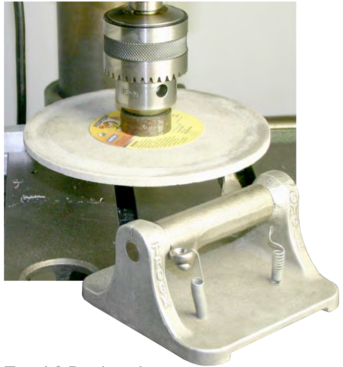
Trock® Rocker Arm Grinding Fixture Use this fixture with a drill press mounted grinding wheel to resurface worn rocker arm pads. Badly pitted rocker arms can be welded using hard-faced rod and re-ground using this fixture. Works with Twin Cam®, Evolution®, Shovel and Sportster® rocker arms. #706-404
