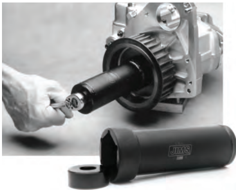
JIMS® Mainshaft Sprocket Nut Socket Heavy-Duty thick wall tube. Extra long two piece design; inner collar supports socket square to nut for safer service work. 1/2" Drive.
