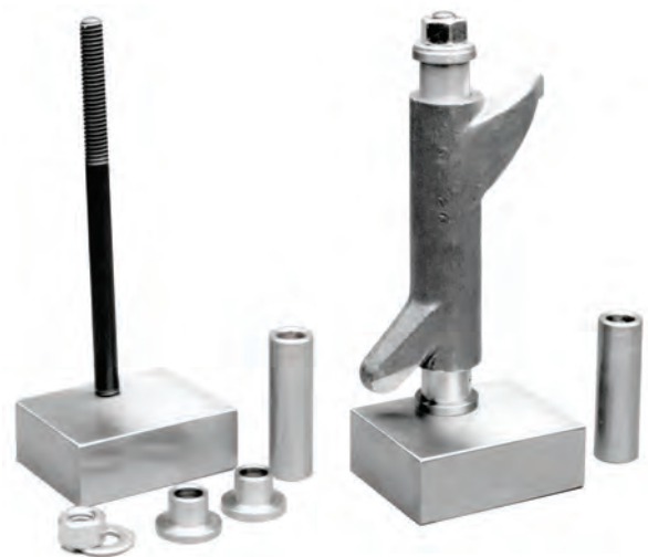
JIMS® Rocker Arm Bushing Installer Use to install rocker arm bushings in rocker arms with or without a press. This tool will install each bushing to the correct depth for the best oil control. Use on all Big Twin 1966-present and Sportster® 1957-present. #758-357
