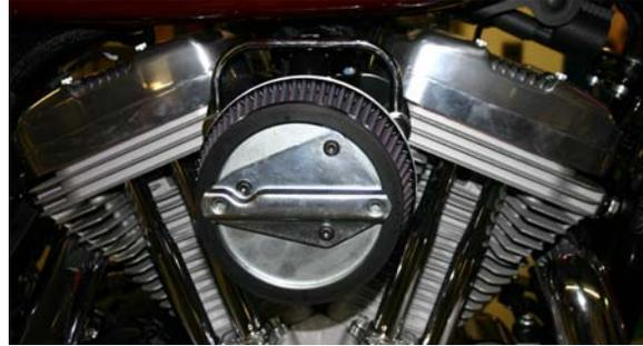
7. Re-install the air cleaner cover using the original mounting hardware (use blue Loctite®). Optional: Use an adhesive to attach the rubber seal trim to the cover for a finishing touch.
