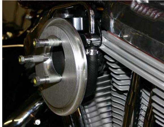
5. Locate the (3) Torx head screws and spacers supplied and Apply blue Loctite® to the screws. Insert a screw through the air cleaner cover bracket, and a spacer over the screw as shown.
