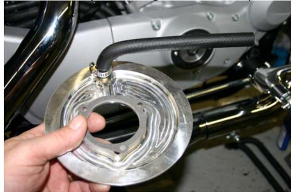
4. Install the gasket to the backplate and install the backplate using the supplied stanchions with blue Loctite®. Attach the backplate hose to the chrome breather tube.
