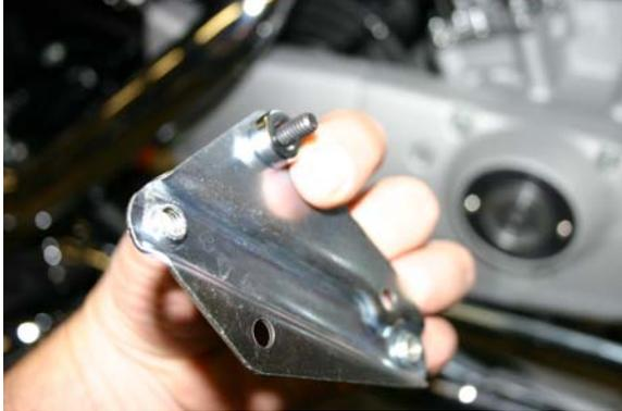
6. Place the filter element over the stanchions and install the cover bracket to the stanchions (the spacer goes between the element and the cover bracket). Leave the first screw loose and install the other two screws with spacers. Tighten the screws.
