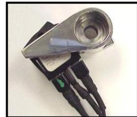
3. Unplug the throttle body harness and install the arming switch over the rear cylinder head throttle body support bracket using the original breather bolt. Install supplied breather spacer to the front head using the other original breather bolt. Re-install throttle body harness with NADS harness routed under T-Body harness plug.
