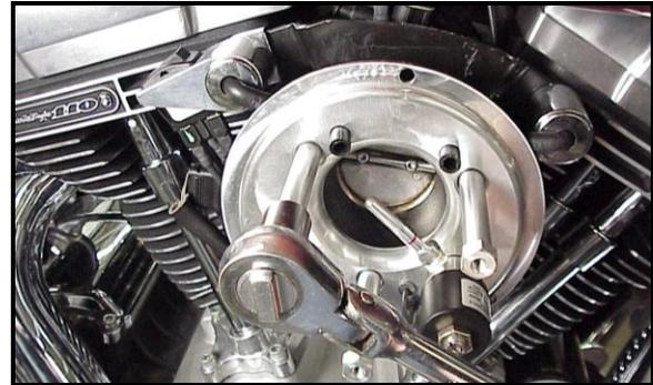
8. Plug two-wire harness connector into NADS solenoid attached to backing plate. Route remaining harness up to frame backbone, under fuel tank to ECM area under seat as shown.
