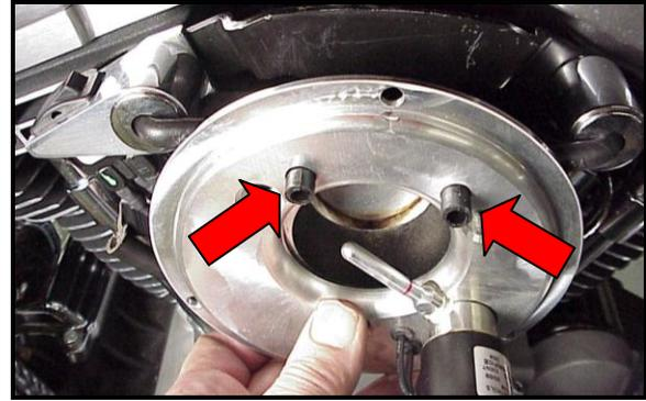
7. Insert supplied gasket between backing plate and throttle body. Apply blue threadlocker to threads of (3) supplied air filter stanchions and install. Tighten stanchions to 120-140 in/lbs.
