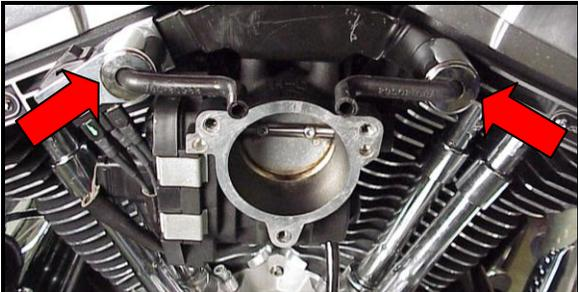
6. Position the NADS backing plate over the throttle body; insert the breather hoses through the two openings in the backing plate as shown.
