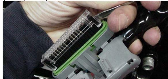
5. Locate positions 9 and 32 on the "wire side" of the connector. On the nitrous harness, insert the terminal of the white w/black tracer wire into position 9 and the terminal of the yellow w/black tracer wire into position 32. Be sure to insert them until they "click" into position and are at the same depth as the other terminals.
