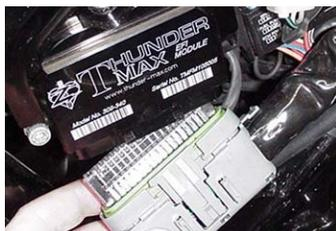
3. Route the NADS electrical harness along the backbone of the motorcycle and position the end of the harness near the ECM.
