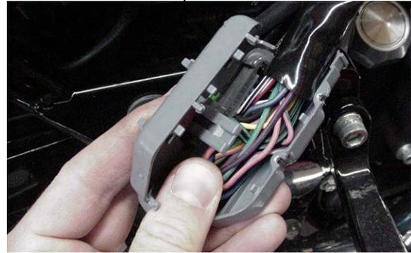
4. Depress the tabs on the connector retainer (clear plastic) and remove it from the connector.
