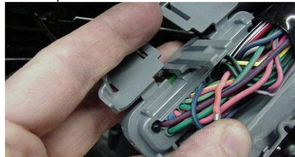
6. Re-install the connector retainer. Position the wires of the nitrous harness so that they exit the strain relief along the same path as the OEM wires. Close the halves of the strain relief around all the wires.
