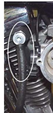
12. Install backplate support brackets over raised bosses in banjo bolts, secure with 5/16-24 socket head screws (do not fully tighten).
