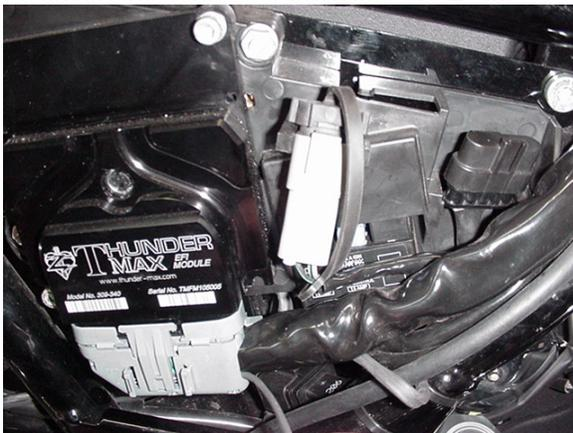
8. Locate the data link connector. Connect the four-position Deutsch connector on the nitrous harness into the data link connector. (If you are also using ThunderMax® AutoTune, you must purchase a Data Plug 'Y' Harness, # 309-343, to run both systems.)
