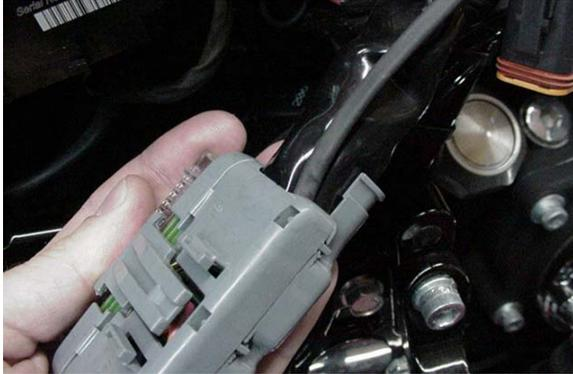
7. Insert the connector back into the ECM.
