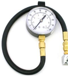
**Fuel Pressure Checking Gauge** Fuel injection systems rely on consistent fuel pressure for proper operation. When fuel pressure drops due to a clogging filter, pinholes in the in-tank fuel line or a faulty fuel pump, performance suffers. This is the FIRST tool you should grab for diagnosis. Quickly installs in-line at the fuel tank outlet and allows you to verify pressure is within spec. **#772-457**
