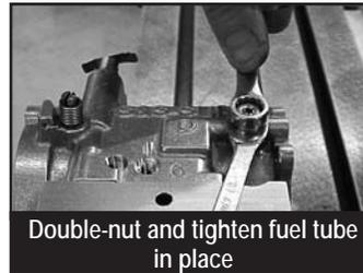
Double-nut and tighten fuel tube in place
