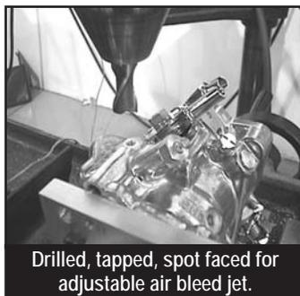
Drilled, tapped, spot faced for adjustable air bleed jet.
