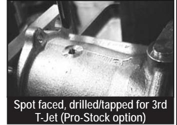
Spot faced, drilled/tapped for 3rd T-Jet (Pro-Stock option)
