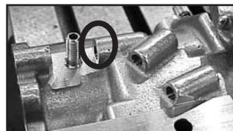
fuel tube hole drilled/tapped, area relieved for T-Jet, fuel tube installed. Circle shows where vent passage should be plugged
