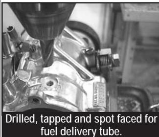
Drilled, tapped and spot faced for fuel delivery tube.
