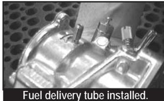
Fuel delivery tube installed.
