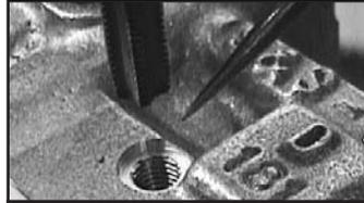
Air bleed passage drilled & tapped for jet.
