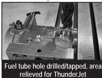
Tapping bowl vent for fitting.
