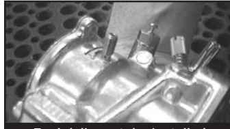
Fuel delivery tube installed.
