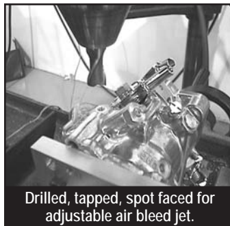
External bowl vent machined in body.
