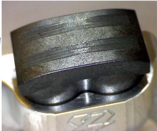
This part has roughly 6,000 miles on it, and is controlling the cam chain very evenly. There are no signs of loss of valve train control on this tensioner! The pressure applied to the chain is even and controlled.
