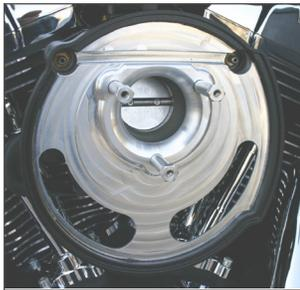
4. Install original breather hose assembly to breather bolt nipples as shown.
