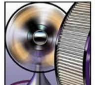
Allow filter to dry. A fan may be used to speed process. DO NOT use heated air blowers, compressed air, or open flame.
