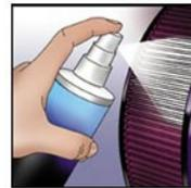
Gently shake off and brush away excess dirt. Spray on Cleaning Solution so that the filter is fully saturated, and let soak for 10 minutes. Rinse filter from the clean side to the dirty side until water comes through. Use only low pressure from a tap or hose.
