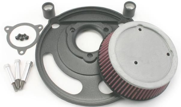
1. Remove existing air cleaner cover, element with cover mounting bracket and plastic backing plate. Do not remove the black head-to-head throttle body support bracket.
