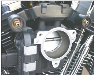
3. Apply a locking agent such as Loctite 242 (blue) to the threads of the (3) stanchions; position the backing plate in position over the throttle body with supplied gasket and start the stanchion threads into the throttle body. Tighten all (3) stanchions to 85-90 inch pounds in a sequence.
