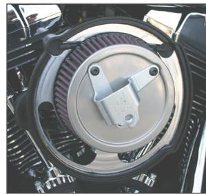
5. Apply low strength threadlocker such as blue Loctite® to (3) Torx head screws provided and install the filter element with original cover mounting bracket to stanchions. Apply threadlocker to original cover mounting screw and re-install factory cover.
