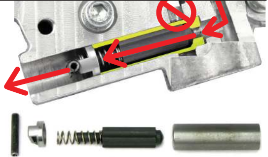
Cam Plate Cutaway with #620-103 Bypass Valve Fluted Design of Needle Allows Oil Flow Through Valve
